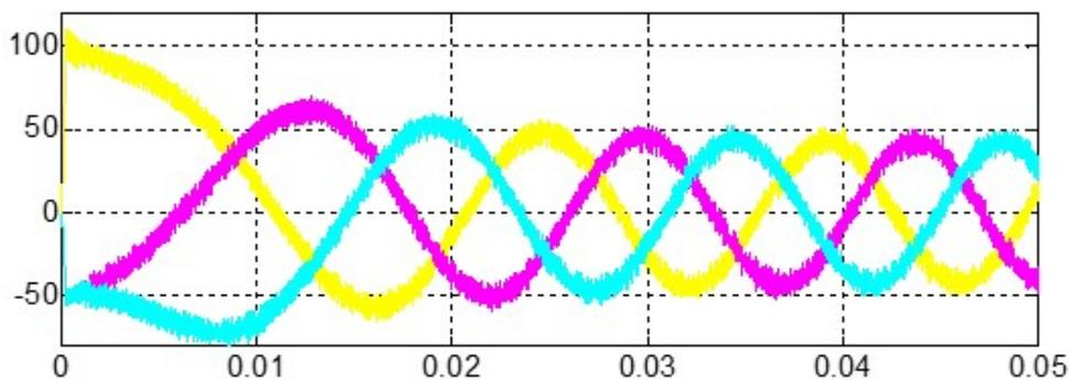
Figure 6. Stator Three-Phase Currents
