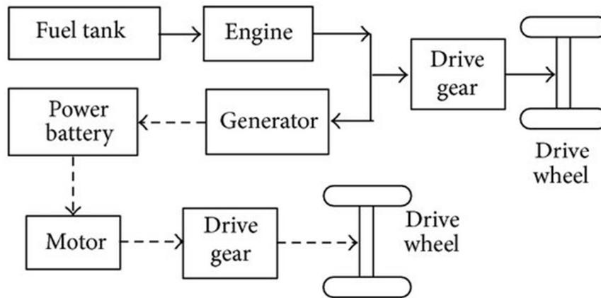
Figure 2. Energy flow diagram
