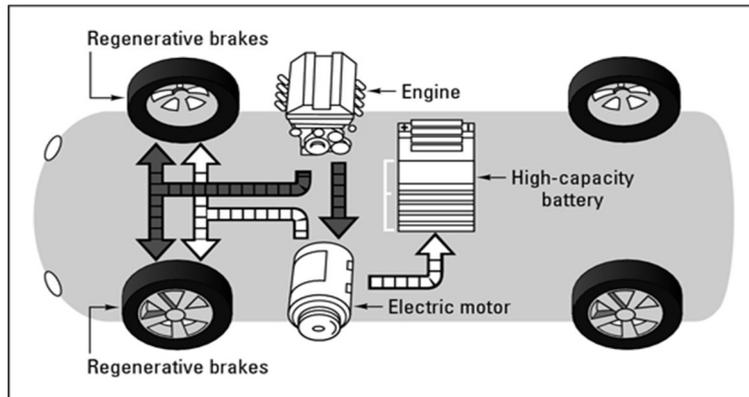
Figure 5. Overview of the motor section
